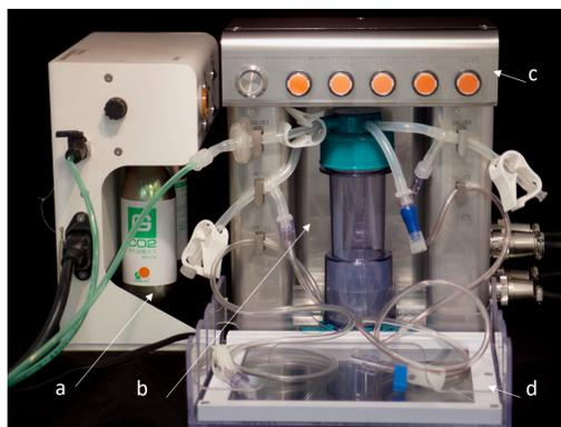
(a) Gas feeder, (b) Culture area, (c) Controller, (d) Glass heater
